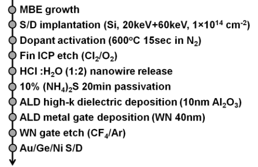
Fig. 2 Fabrication process flow for vertically stacked InGaAs GAA nanowire MOSFETs.
